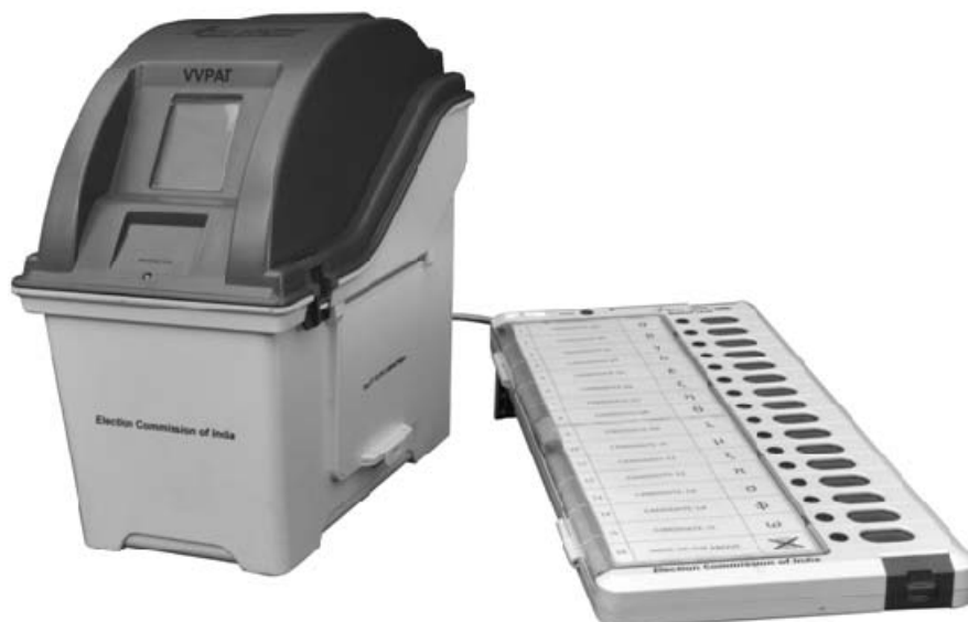
Figure 3.8 - Relative Placement of BU and VVPAT - M3
