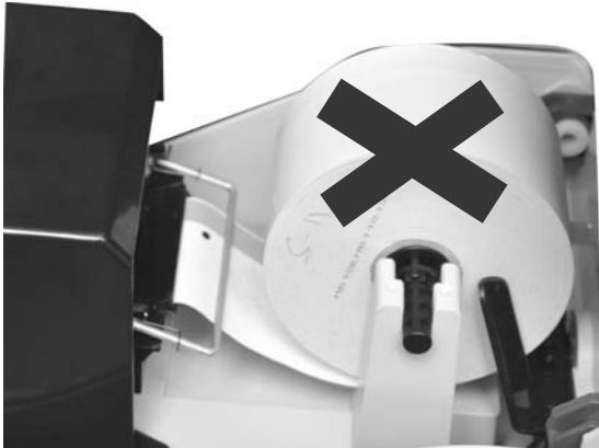
Figure 3.13a - Improper Paper Insertion
